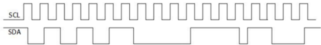
Figure 14.4 Schematic diagram of I2C serial bus
