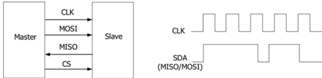
Figure 14.5 SPI Bus Schematic
