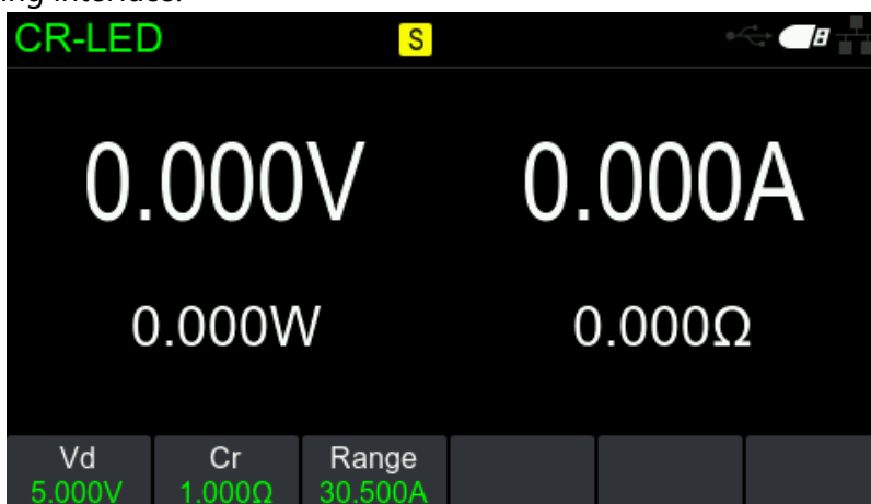
Figure 6-5 CR-LED test function
