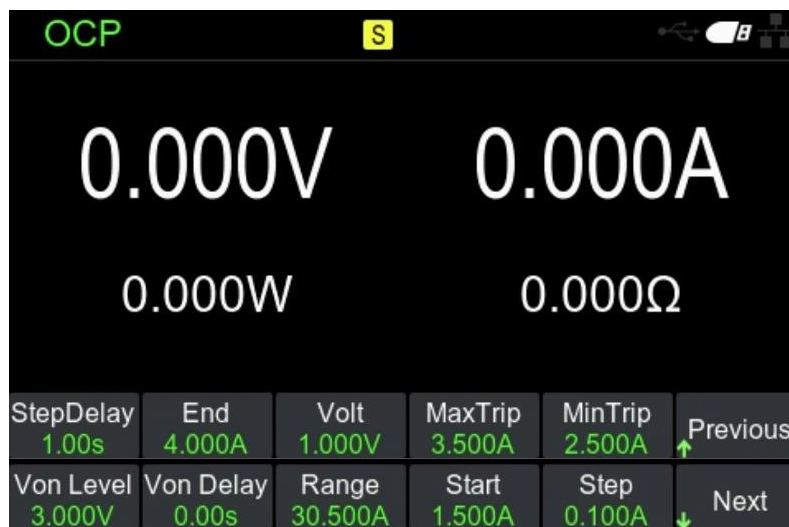
Figure 6-1 OCP test function
