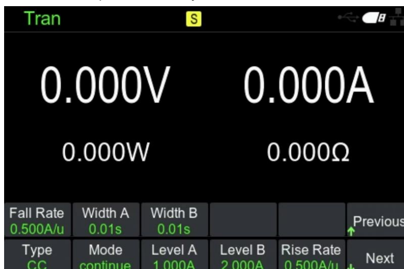
Figure 6-9 Continuous mode setting interface
